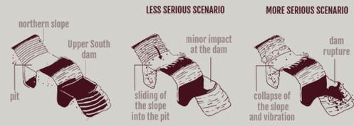
Scenarios of instability of the slope and dam structure. Source: G1. 31/05/19.
